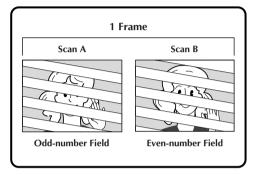
Records 30 odd and 30 even image Fields, for a total of 60 per second. Since there is a time lag between an odd and even Field, when they are combined to make 1 Frame the part of the image that is moving appears as image jitter. However, during normal playback, the moving picture looks smooth and natural.
